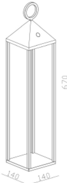
Beautiful outdoor lamp for long summer nights! The fixture is produced in die-cast aluminium and powder coated to last outdoors. 9 hours work time and 5-7 charge time operated by 2 x 220mAh lithium battery. Dimmable by touch switch to create the atmosphere you'd like.
