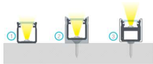
The result of installation of profile Y with BASIC cover, using (1) a double-sided tape, (2) a mounting clip Y, (3) an assembly profile Y M1 and a metal mounting clip Y
