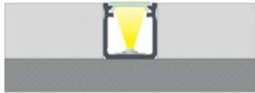
The end result of installation of recessed profile Y with BASIC cover between two plasterboards
