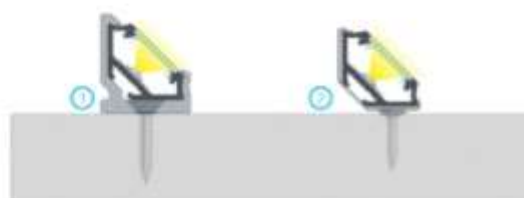
The end result of assembly of corner profile C with a BASIC cover using using (1) plastic mounting clip CH, (2) metal mounting clip CH
