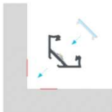
Installation manual for C profile with BASIC cover using double-sided tape
