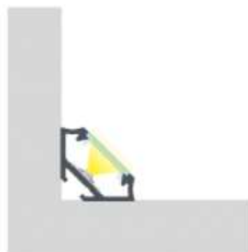
The end result of assembly of corner profile C with a BASIC cover using double-sided tape
