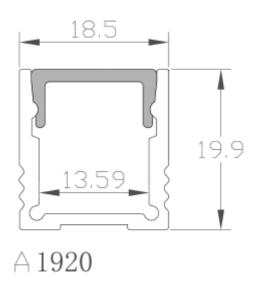
Anodized Aluminum profile for surface mounting. Includes opal cover, 2pcs end cap, 2pcs end cap with hole for cable and mounting clips.
