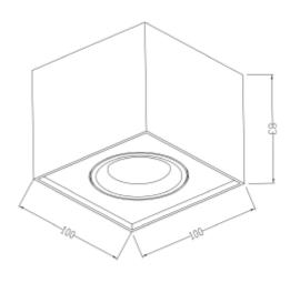
Cobra 360° Rotatable Surface is a flexible surface mounted downlight developed from our vast experience with earlier models. The 360° Rotatable light head makes it possible to tilt the light beam up to 25 degrees in all directions.
